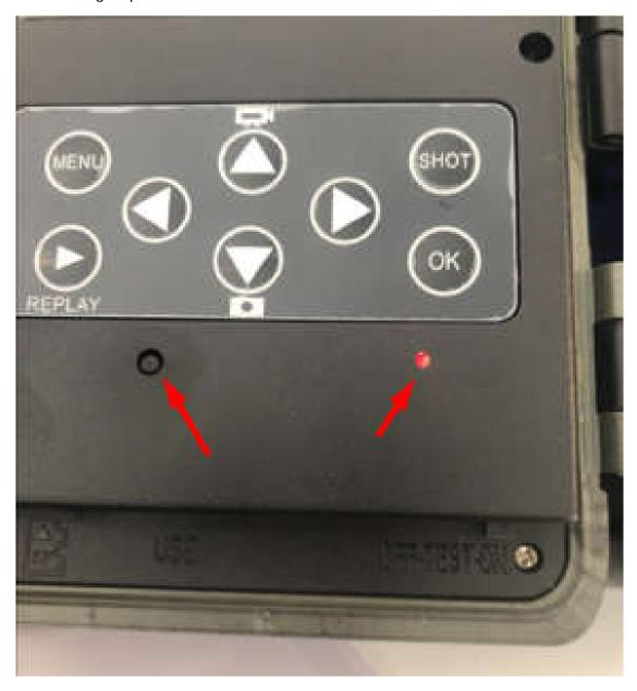
2. Then push the remote control once, and the red diode on the camera will turn off again. Now the remote are paired.
