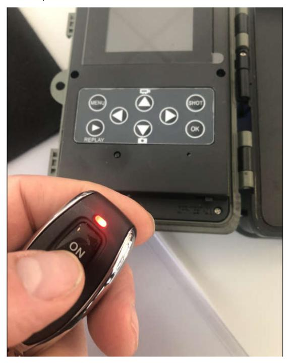
When you have the camera in ON mode you can use the remote to turn on Wi-FI on the camera. Then you can use the smartphone to see what photos are on the camera + do some settings.
